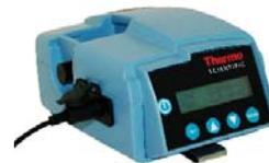
PM-205 Particulate Meter (may be bracketed to side of security case)
