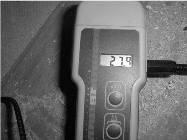
Figure 2. In this case water from the ground has passed through the concrete slab up to the wooden sill laying on top of the concrete without any moisture barrier between. The reading is close to the fibre saturation point in pine (28%).
