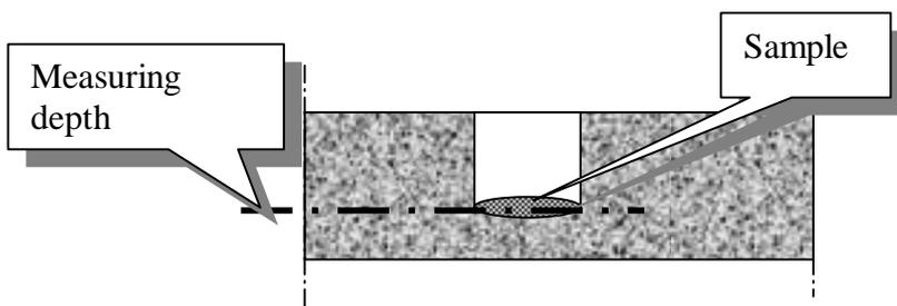
Figure 7. The sample has to be taken out as close as possible to the depth you are interested in.
