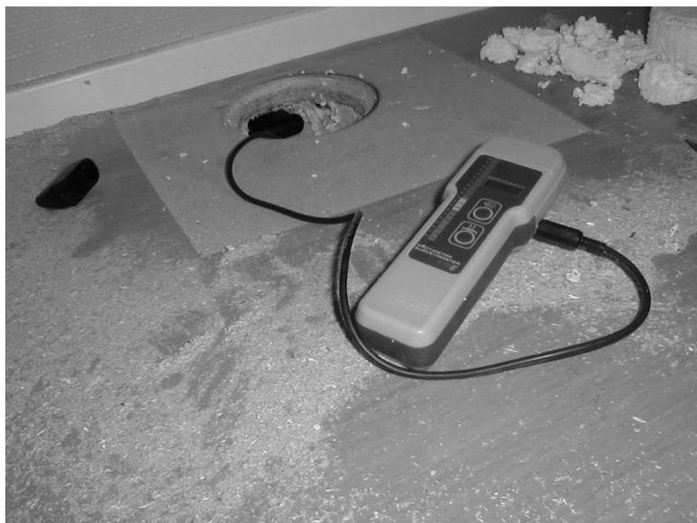
Figure 1. Two nails are pushed in to the wood. The nails are connected to the instrument by a cable. It is possible to use loose nails if it is too tight where you are going to measure. The electrical power gives a higher reading on the display if the moisture content is high. The same method can be used in other porous materials to indicate where the moisture content is high.
