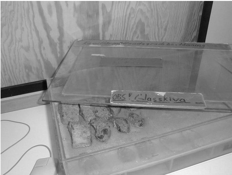
Figure 4. In the laboratory the sample is taken out from the plastic bags and weighted carefully. The samples are placed in a tight box made of transparent plastic or glass on a metal net just in contact with water
