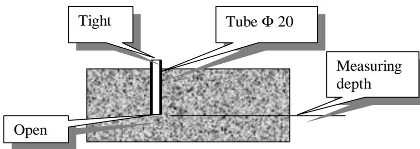
Figure 6. In concrete you can drill a hole  $\Phi$  20 mm down to the level of interest and seal it inside with a plastic tube open in the bottom or with equipment delivered together with some RH instruments. The measuring can be done one week after the drilling and preparation of the hole is done.
