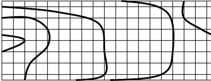
Figure 5. Scanning on floors searching for high readings often give a good picture over the differences in moisture content in different parts of the floor. Indicating at every 500 mm over the floor make it possible to do a drawing telling where to measure and sometimes the possible reason to the high moisture content. High readings close to a bathroom wall indicate leakage from that direction.
