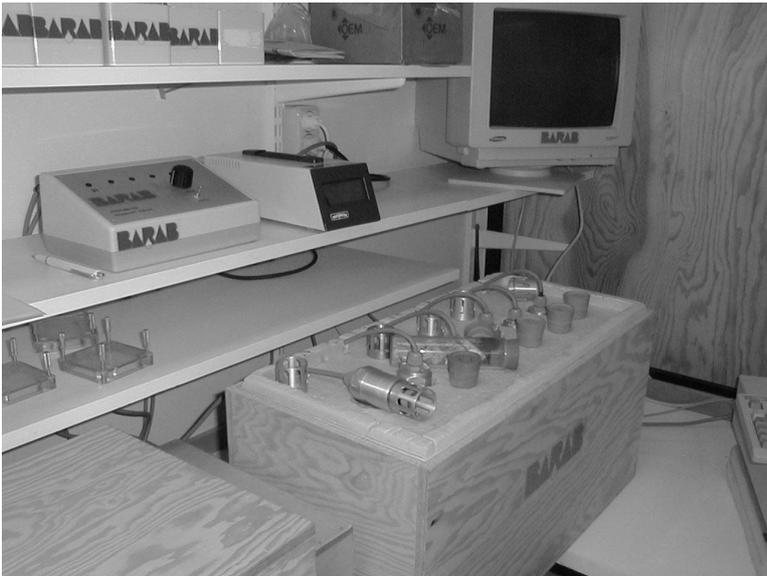
Figure 8. It is important to keep a constant temperature in the samples during measuring. On the picture you can see a thermal insulated box containing six measuring boxes.
