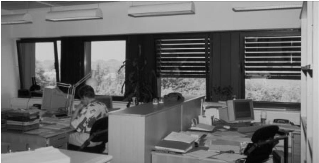
**Figure 6: Solar shading in the offices is exterior Venetian blinds.**
