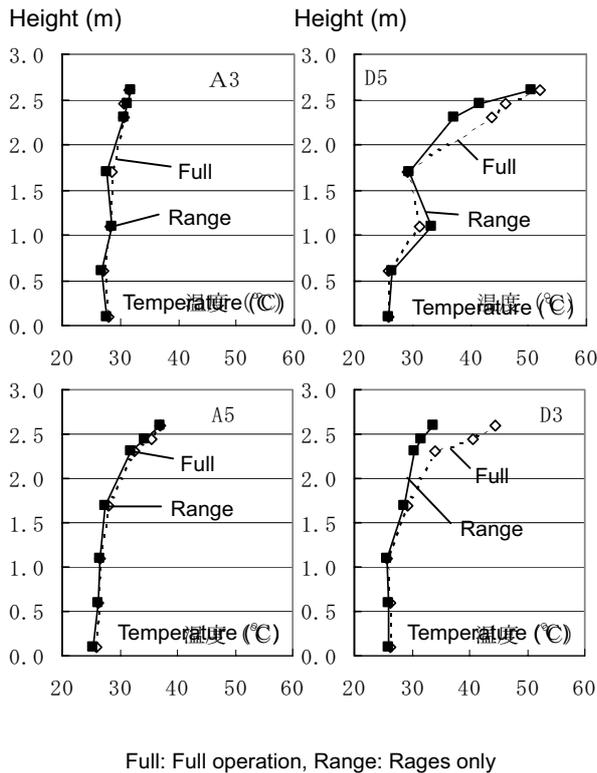
Figure 1 Vertical temperature distribution by precise measurement
