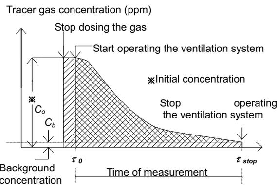
Figure 3 Concept of the sampling bag method
