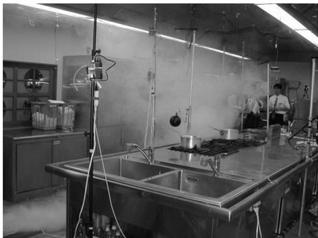
Figure 5 Visualization with smoke
