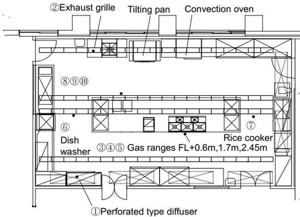
Figure 2 Points of measuring tracer gas concentration
