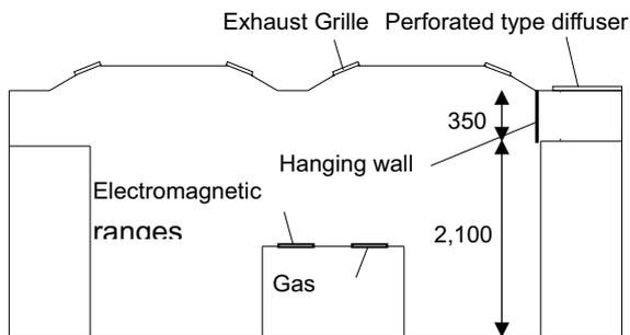
Figure 4 Installation of a hanging wall
