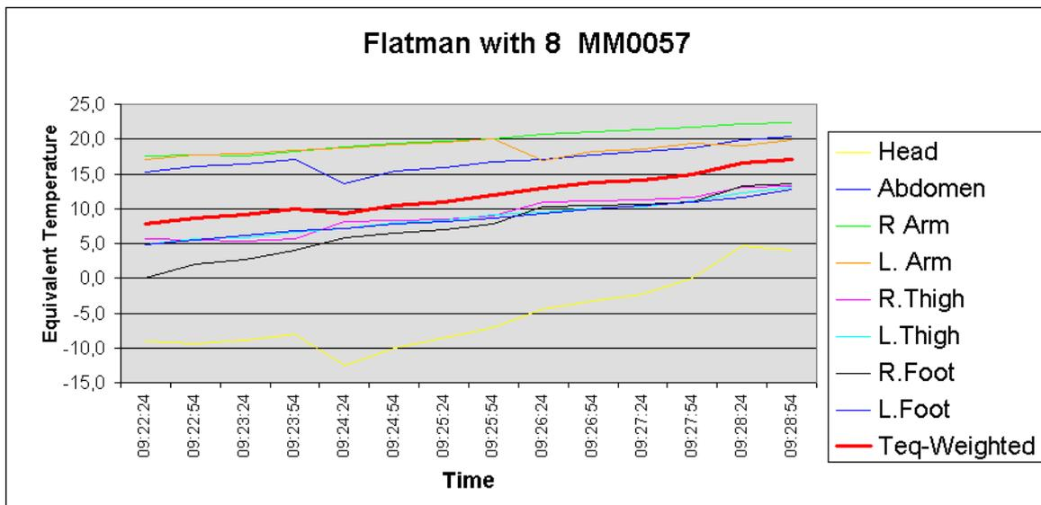
Fig.4 Measurement of Equivalent Temperatures during a warm-up experiment in a vehicle
