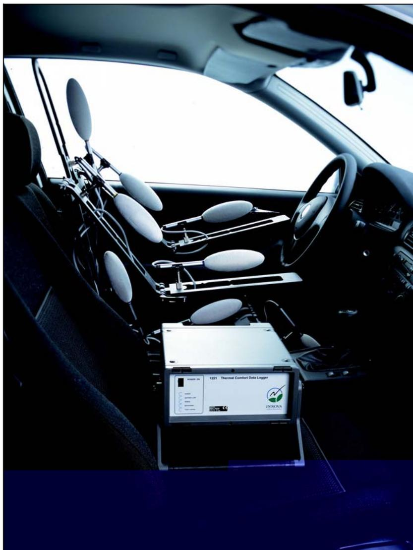
Fig.1 Flatman and the Thermal Comfort Data Logger 1221
