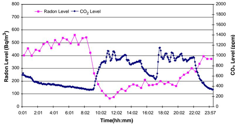
Fig. 7. Typical radon and CO<sub>2</sub> profiles in the lecture theatre while using dual mode demand control ventilation strategy.
