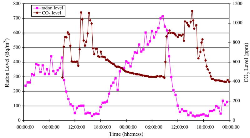
Fig. 3. Typical radon and CO<sub>2</sub> profiles in the lecture theatre while using CO<sub>2</sub> based demand control ventilation.
