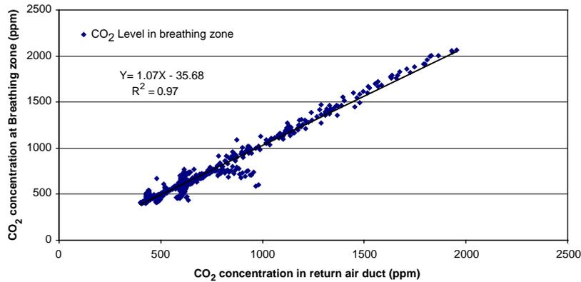
Fig. 4. Correlation between the CO<sub>2</sub> concentration at breathing zone and in return air duct.
