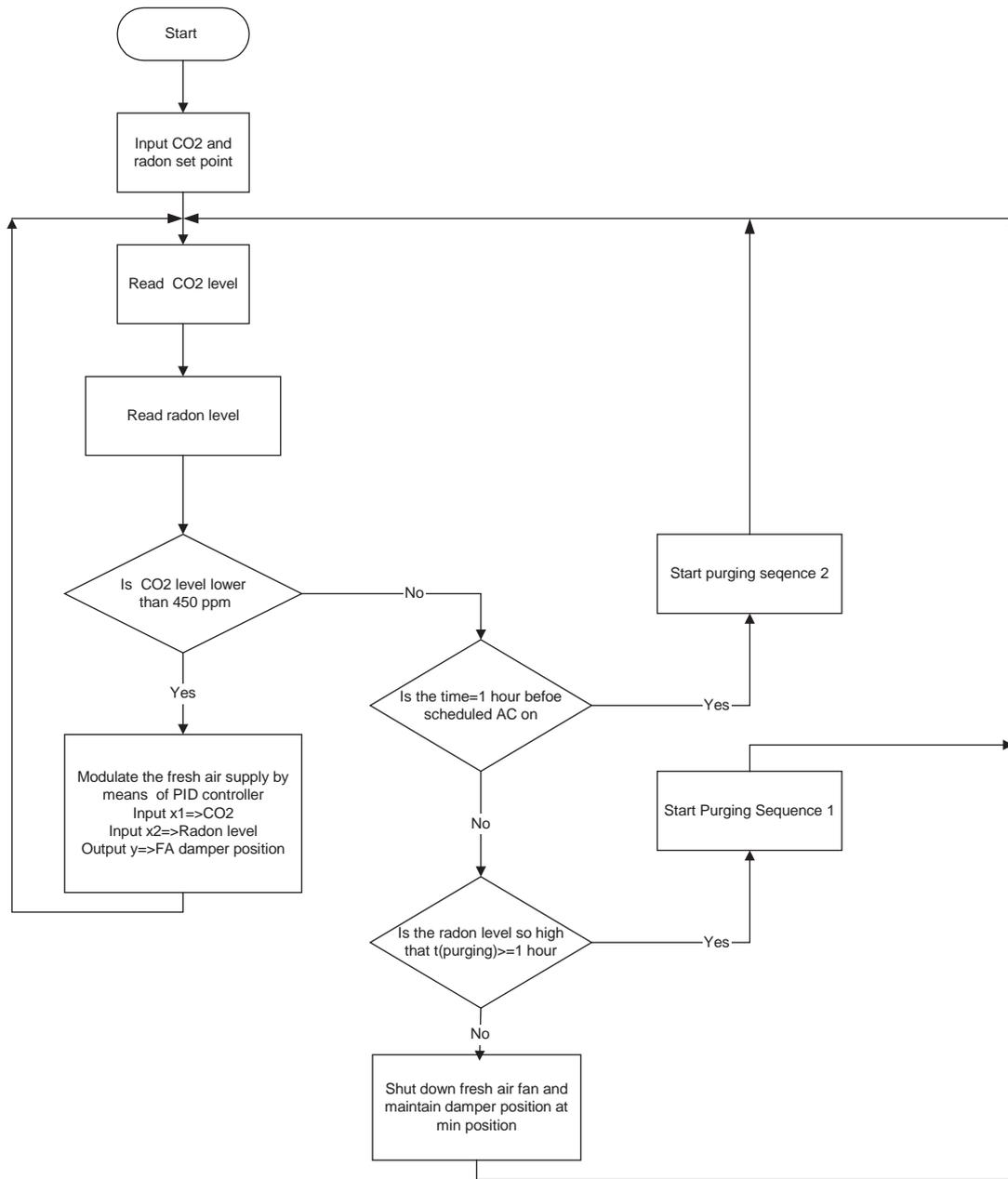
Fig. 5. The flow chart of the CO<sub>2</sub> and radon based demand control ventilation strategy.
