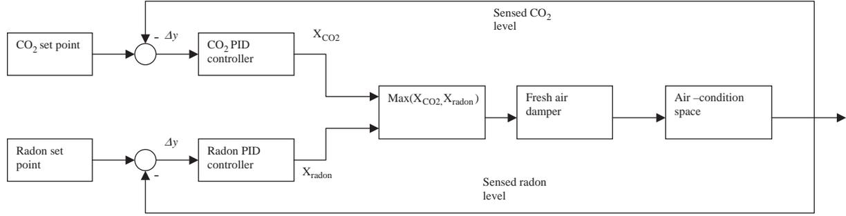
Fig. 6. Flow chart of the modulation mode.
