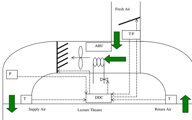
Fig. 1. Schematic diagram of the HVAC system serving the lecture theatre.
